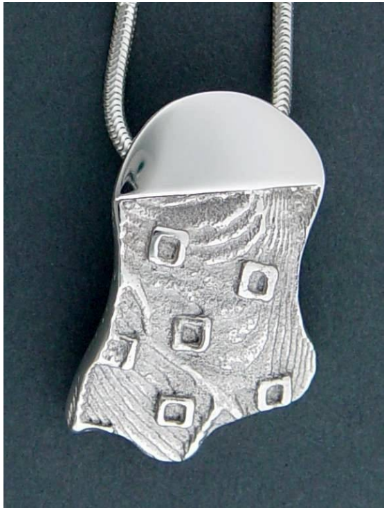
Casting in cuttlebone
